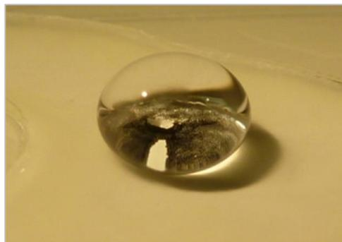
*Super-hydrophobic microstructured surface
